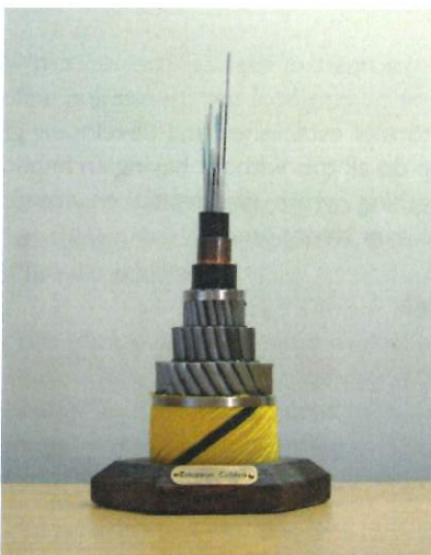
Section of a submarine cable,
